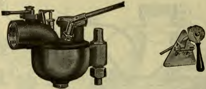
FIG. 166.—A Surface Carburettor, arranged for dashboard control of fuel needle valve. A universal joint is fitted to the valve stem having an extension connecting with the graduated dial, shown at the right.
